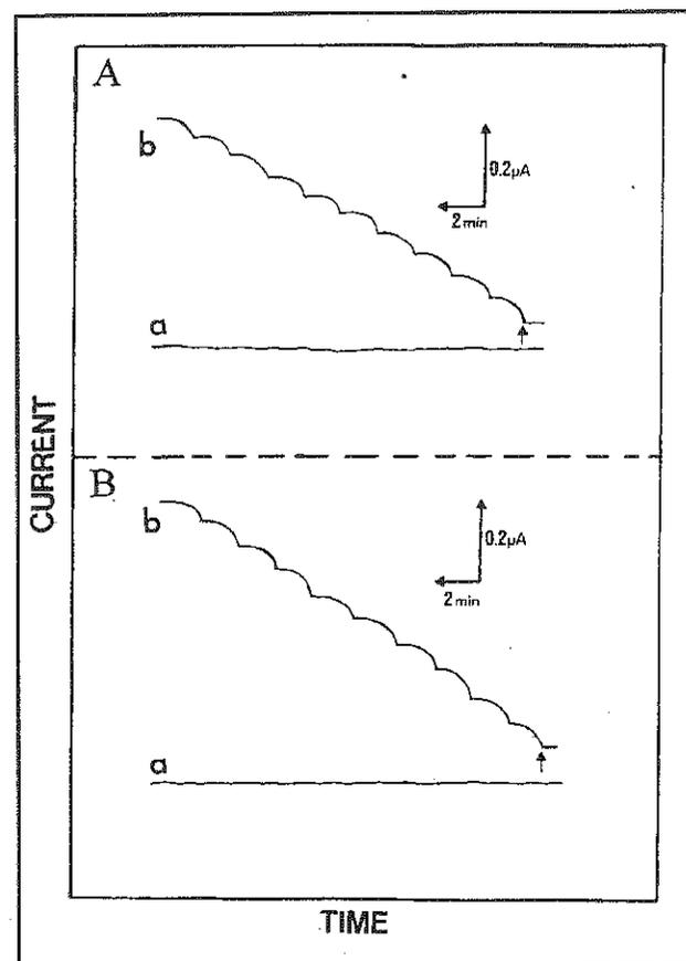
Figure 2. Amperometric response for successive additions of  $3 \times 10^{-5}$  M dopamine (A) and phenol (B) at the ordinary (a) and mushroom tissue based (b) carbon paste electrodes. Other conditions as in Fig. 1.
