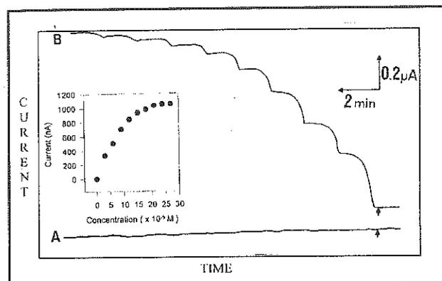
Figure 1. Current-time recording obtained at (A) the plain and (B) 5% mushroom tissue (w/w) containing carbon paste on increasing the concentration of catechol in  $3 \times 10^{-5}$  M steps. Batch experiment, stirring the solution at 400 rpm and  $-0.24$  V operating potential. Solution 0.05M phosphate buffer (pH 7.4) containing 10 mM  $K_4Fe(CN)_6$ . Also shown (inset) is the resulting calibration plot for the modified electrode.
