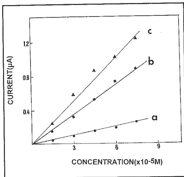
Figure 5. Effect of mushroom content in the carbon paste on the phenol response. Mushroom loadings 5 (a), 10 (b), 15 (c) % (w/w) for carbon paste with  $6 \times 10^{-5}$  M phenol increments. Other conditions as in Fig. 1.
