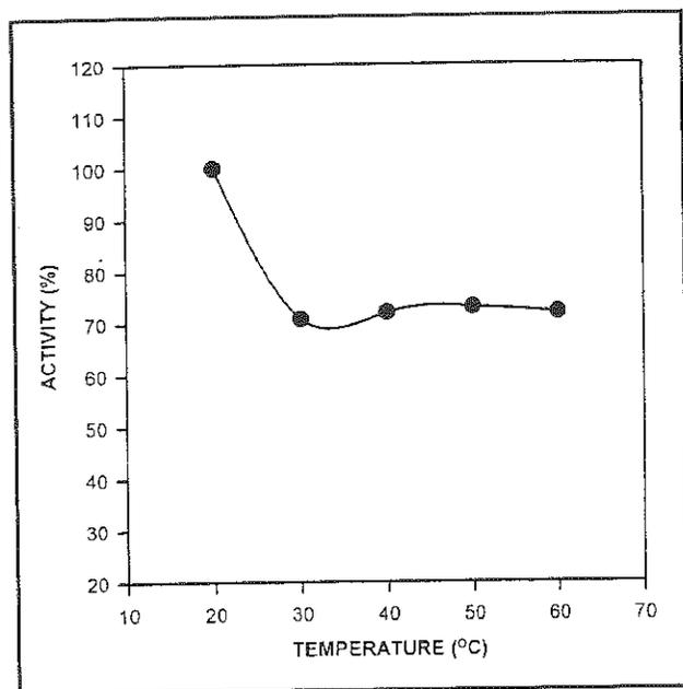
Figure 4. Dependence of the  $5 \times 10^{-3}$  M phenol response on the operating temperature. Other conditions as in Fig. 1.
