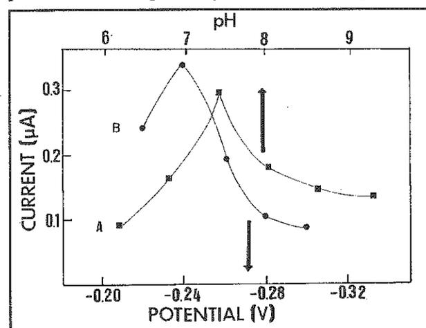
Figure 3. Dependence of the  $5 \times 10^{-3}$  M phenol response on the solution pH (A) and operating potential (B) respectively. Other conditions, as in Fig. 1.
