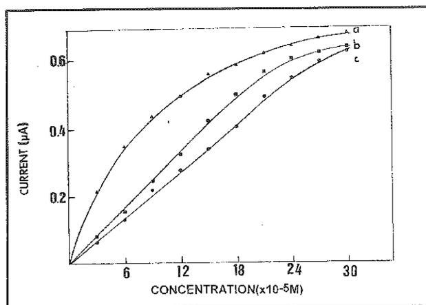
Figure 7. Dependence at the steady state current on the concentration of (a) catechol, (b) dopamine and (c) phenol, I vs. C. Other conditions as in Fig. 1.
