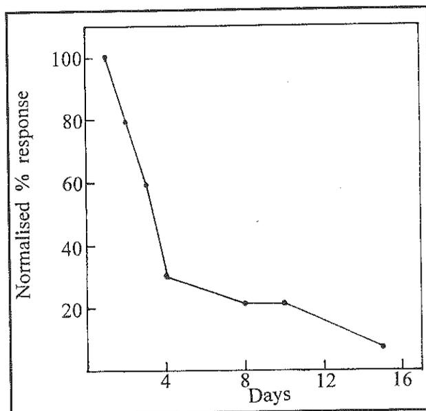
Figure 6. Stability of the response to  $1.5 \times 10^{-5}$  M phenol. Other conditions, as in Fig. 1.
