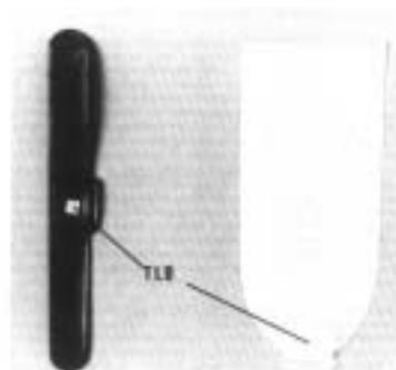
**Figure 2.** Thermoluminescent Dosimeter TLD<sup>2</sup>. Left: TLD incorporated into plastic strip; Right: TLD attached at the end of a finger stall.
