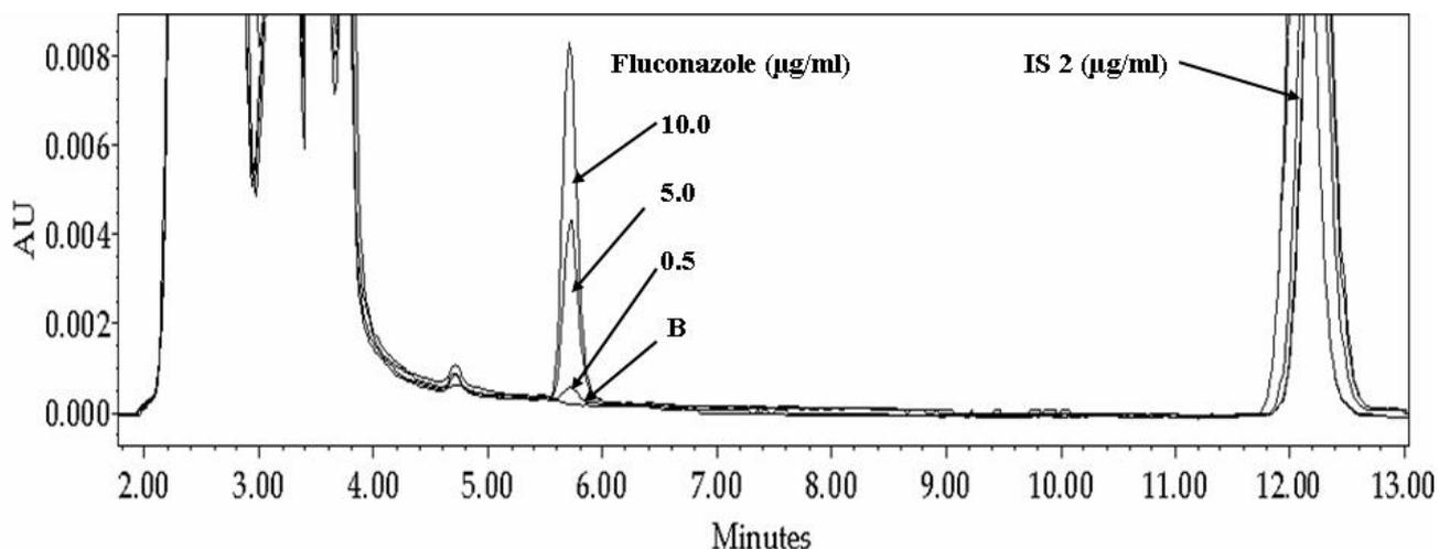
**Figure 1.** Overlay of chromatograms of blank human plasma (B) spiked with 0.5, 5.0, or 10.0 µg/ml of fluconazole and 2.0 µg/ml acetophenetidin (internal standard, IS).
