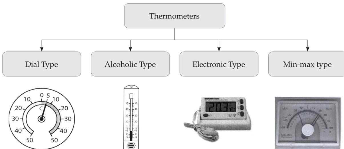
Figure 6. Different types of thermometers (12).
