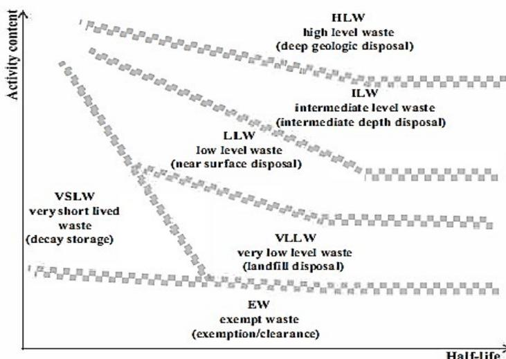
**Figure 1.** Classification of radioactive wastes (Policies and Strategies for Radioactive Waste Management, 2009)
