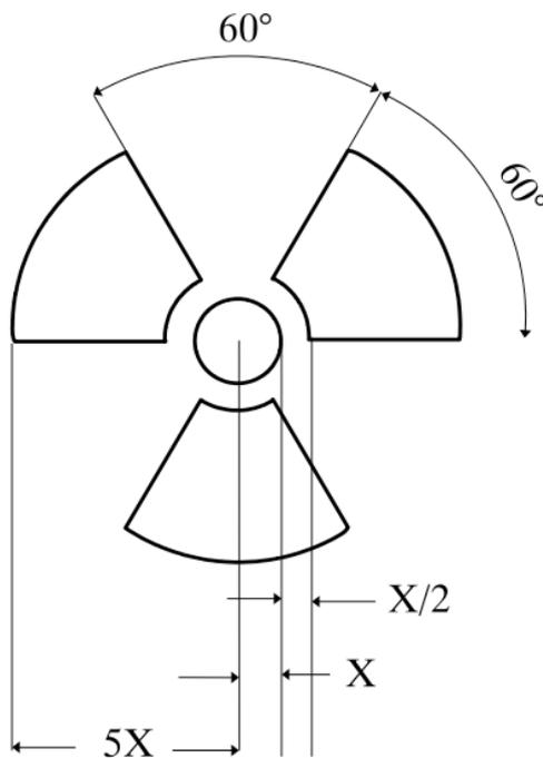
**Figure 2.** Radiation Symbol (The smallest value for X is 4 mm)
