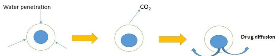
**Figure 5.** Gas generation of a solid core coated by effervescent layer after placing in water.
