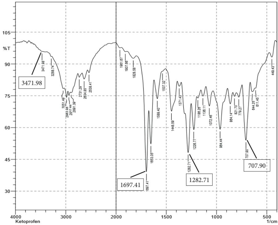
Figure 11: FTIR spectrum of ketoprofen pure drug
